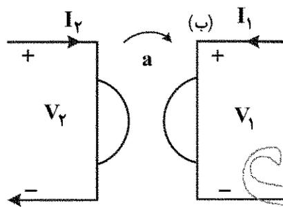
$V_1 = aI_2, V_2 = -aI_1$
