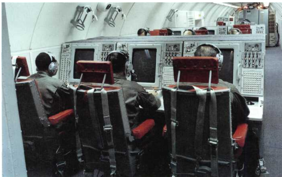
One of the most vital aspects of modern air combat is real time intelligence. An air arm without an airborne warning and control system (AWACS) simply won't be able to defend its airspace for long against a well trained foe who has this capability. Our photo depicts the radar plotting control centre aboard a Boeing E-3 Sentry, the most sophisticated AWACS platform in service and presently in the inventories of USAF, NATO, Saudi Arabia, France and Britain. (Boeing)
